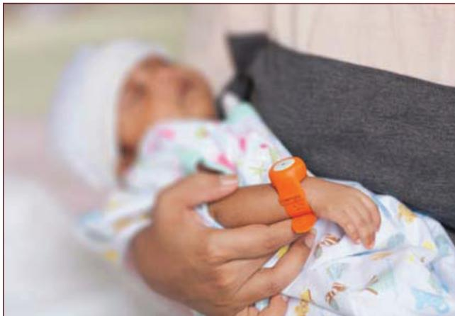
**[Table/Fig-1]: The BEMPU Hypothermia Alert Device (TempWatch).**
